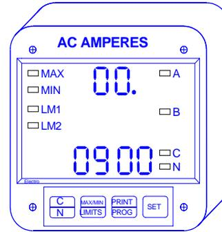
⇒ Once the entry is complete, the new value is displayed in the lower level, the middle level is blank and the group and function number are displayed in the upper level.
