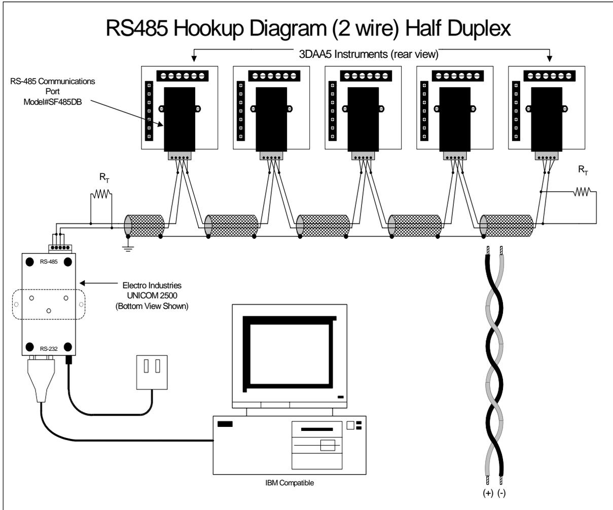
**Figure 4.2:** 2-Wire RS485 Communication Hookup Installation Half Duplex
