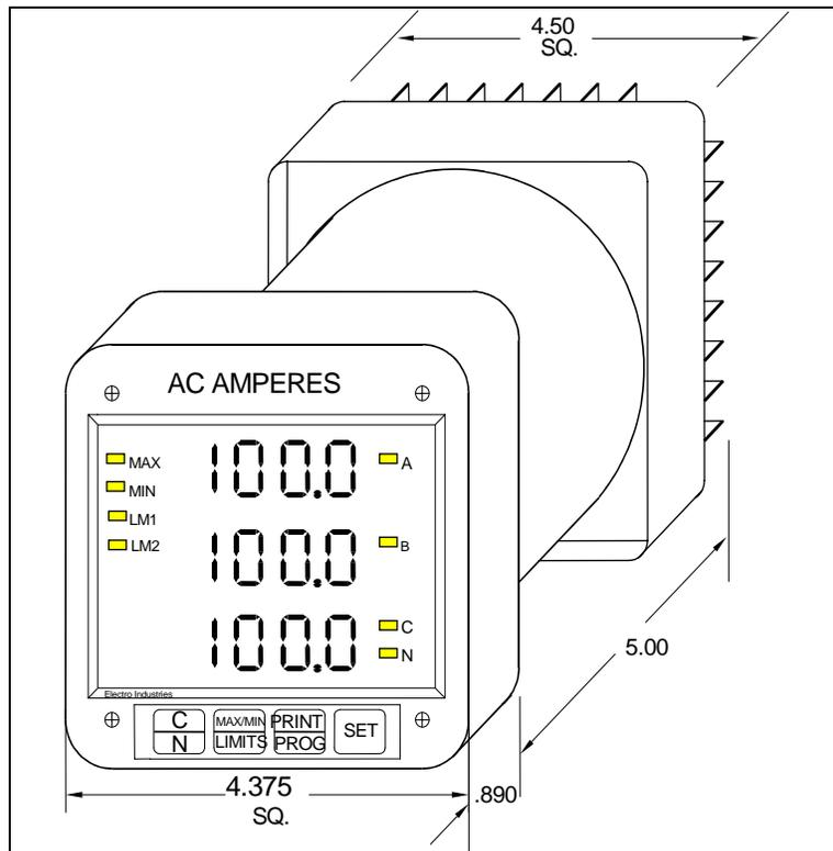
Figure 2.2 Standard Installation of the 3DAA5
