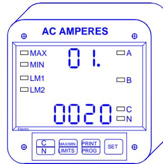
⇒ Once the entry is complete, the new value is displayed in the lower level, the middle level is blank and the group and function number are displayed in the upper level.
