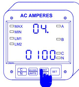
⇒ Once the entry is complete, the new value is displayed in the lower level, the middle level is blank and the group and function number are displayed in the upper level.
