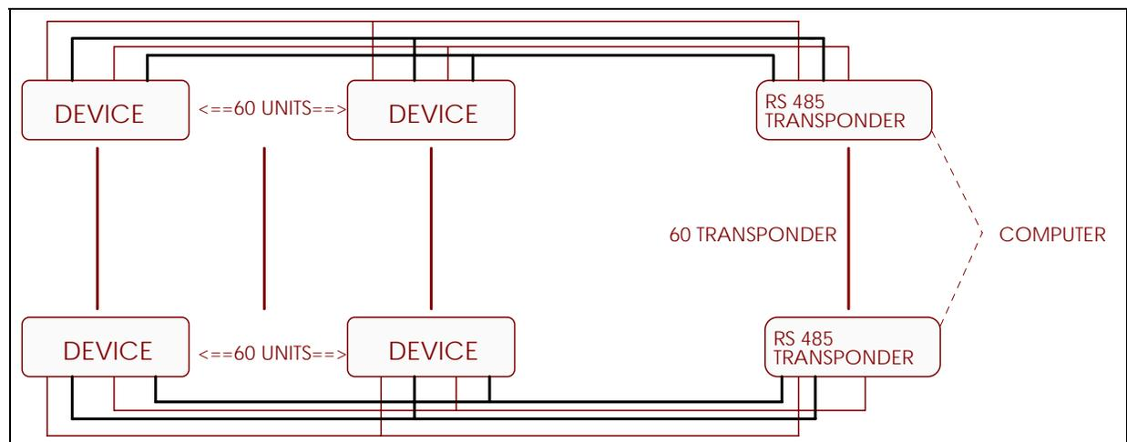
**Figure 4.7** 4-Wire RS485 Communication Installation Hookup with Transponder
