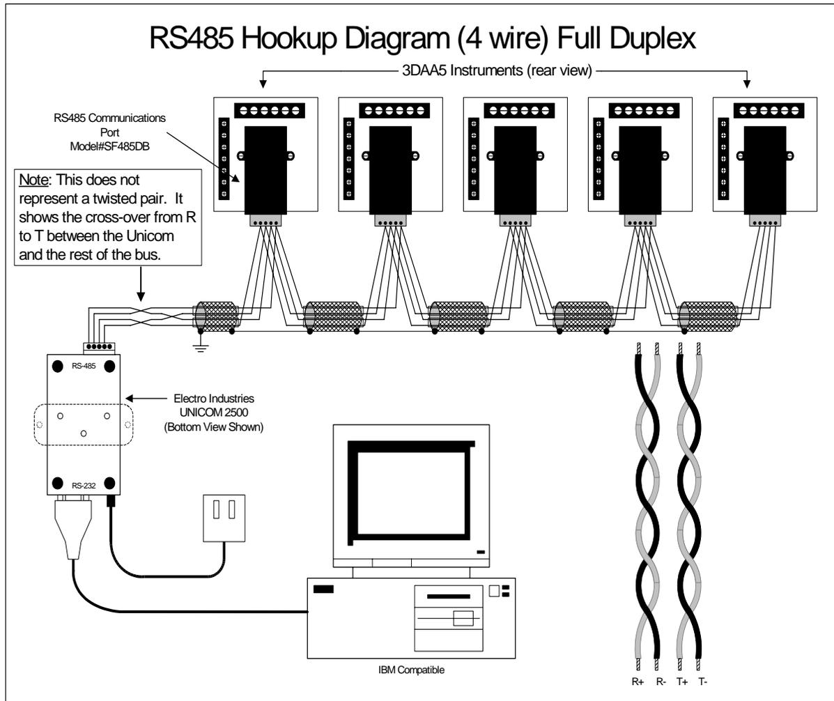
**Figure 4.4:** 4-Wire RS485 Communication Hookup Installation Full Duplex
