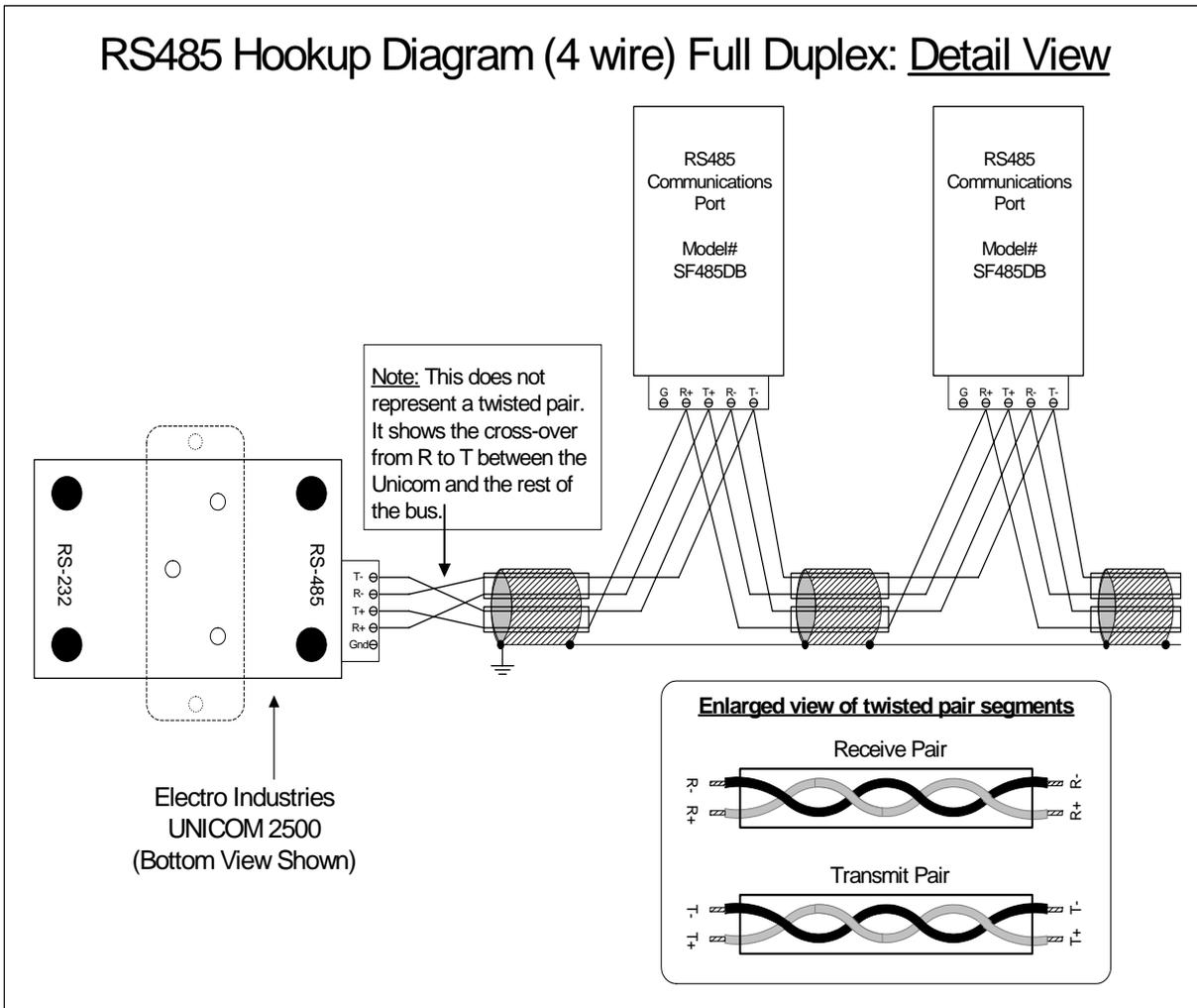
**Figure 4.5:** 4-Wire RS485 Communication Hookup Installation, Full Duplex, detail view
