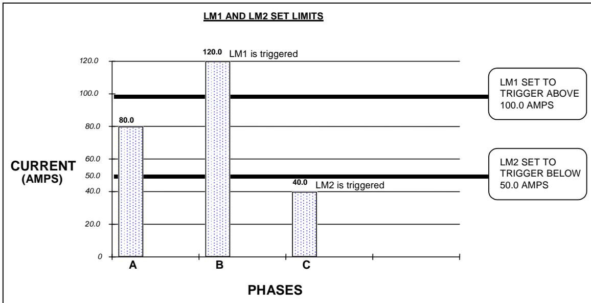
Figure 11-1: Example of LM1/LM2 Set Limits
