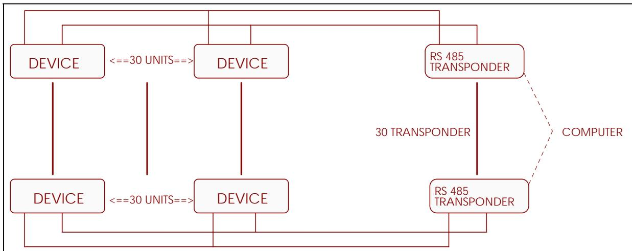
**Figure 4.6** 2-Wire RS485 Communication Installation Hookup with Transponder
