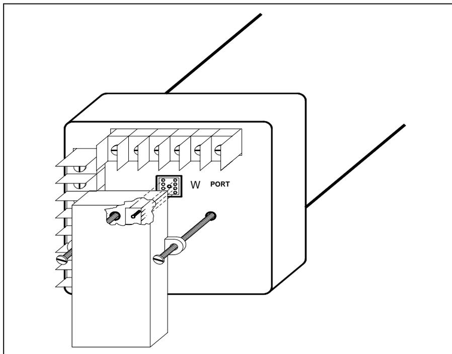
Figure 2.4: Optional Communication Converter or DC Output Module Installation
