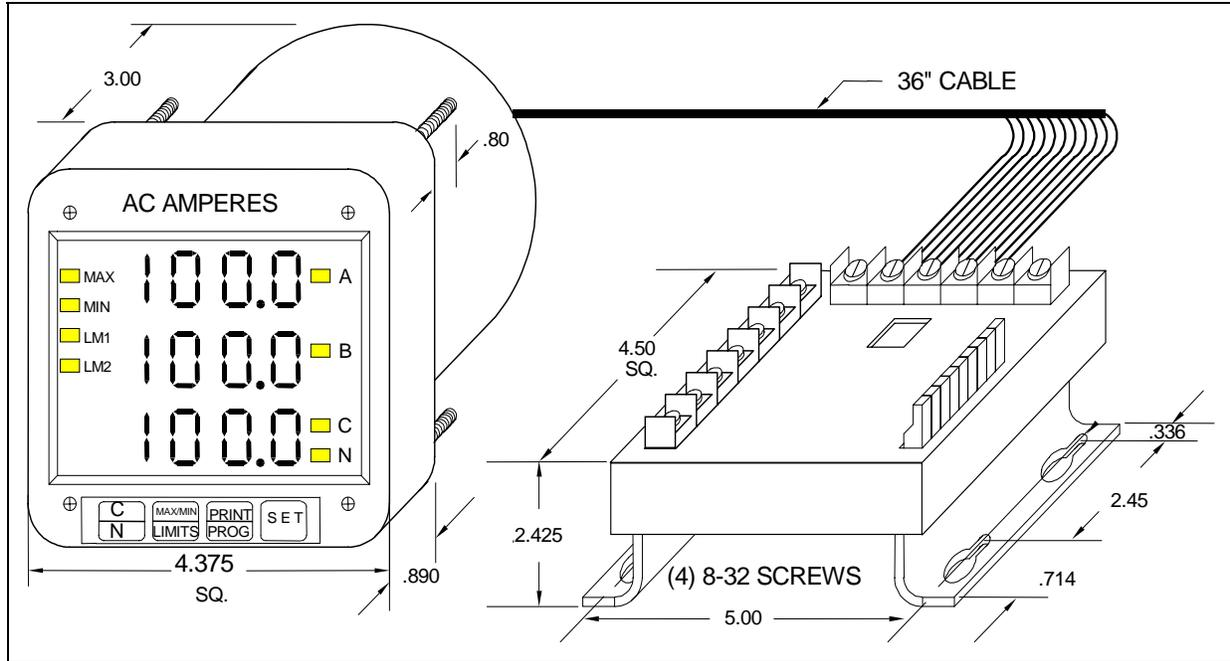
Figure 2.1 Installation of the 3DAA5 meter with K-110 Option for limited space conditions
