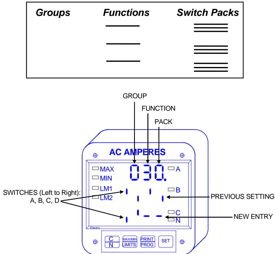
**Figure 6.1:** The Programming Mode, showing Group 0, Function 3, PACK 0 and its switch settings
